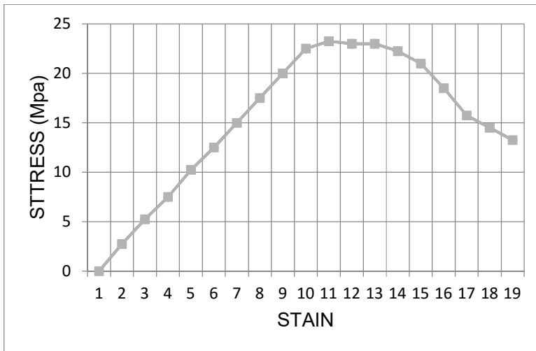
Fig. 2 Shear test graph (test along fibre grain) V_f = 10\%
